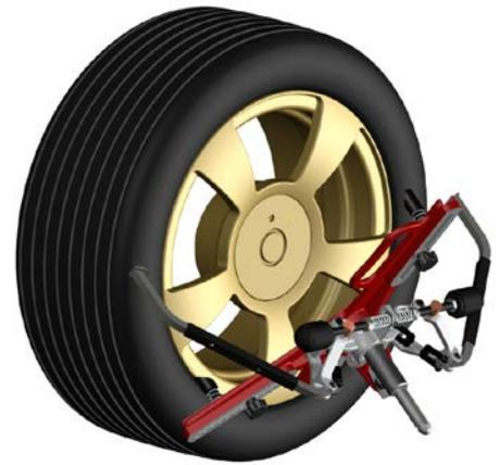
Check if all three feet fit the base of the rim perfectly, if necessary correct the presetting with the star grip screw.
