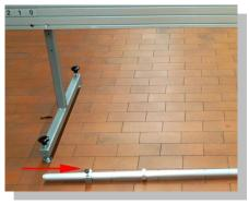
Step 3 Move the tube clamps to the centre. Reattach the centre bar.
