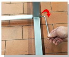
Step 2: Slide the tube clamps on the centre bar left and right
