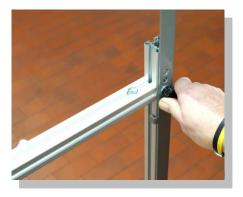
STep 7 Slightly loosen all 3 plastic screws, hook in the reflector panel and tighten plastic screws hand tight only.
