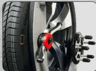
The ergonomically positioned clamping and centering tools can be removed from the holder in one swift movement.
