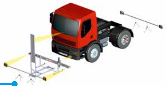
The measuring crosshead and calibration reflector are aligned horizontally at an exact distance in front of the vehicle.
