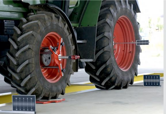
Toe alignment in modern tractors and agricultural machinery is as important as in cars and utility vehicles.
