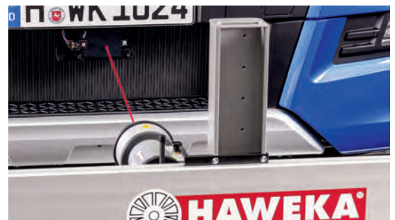
SAD4000 camera setting on the ACC sensor
